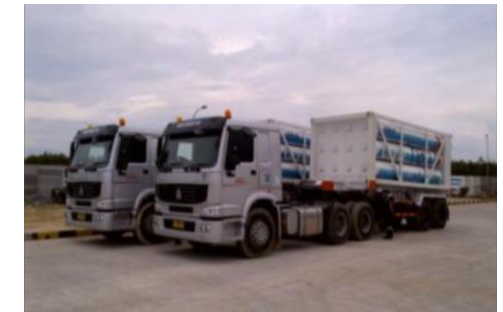
Gas Transport Mobile CNG Cylinder Tube
